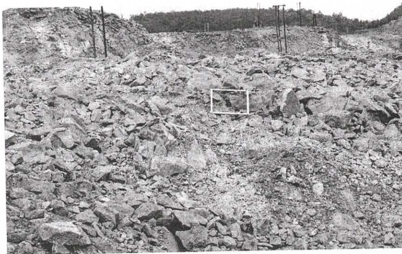
View of the blasted muck resulted due to shovel bench blasting at Nigahi Project, NCL — MT/164
