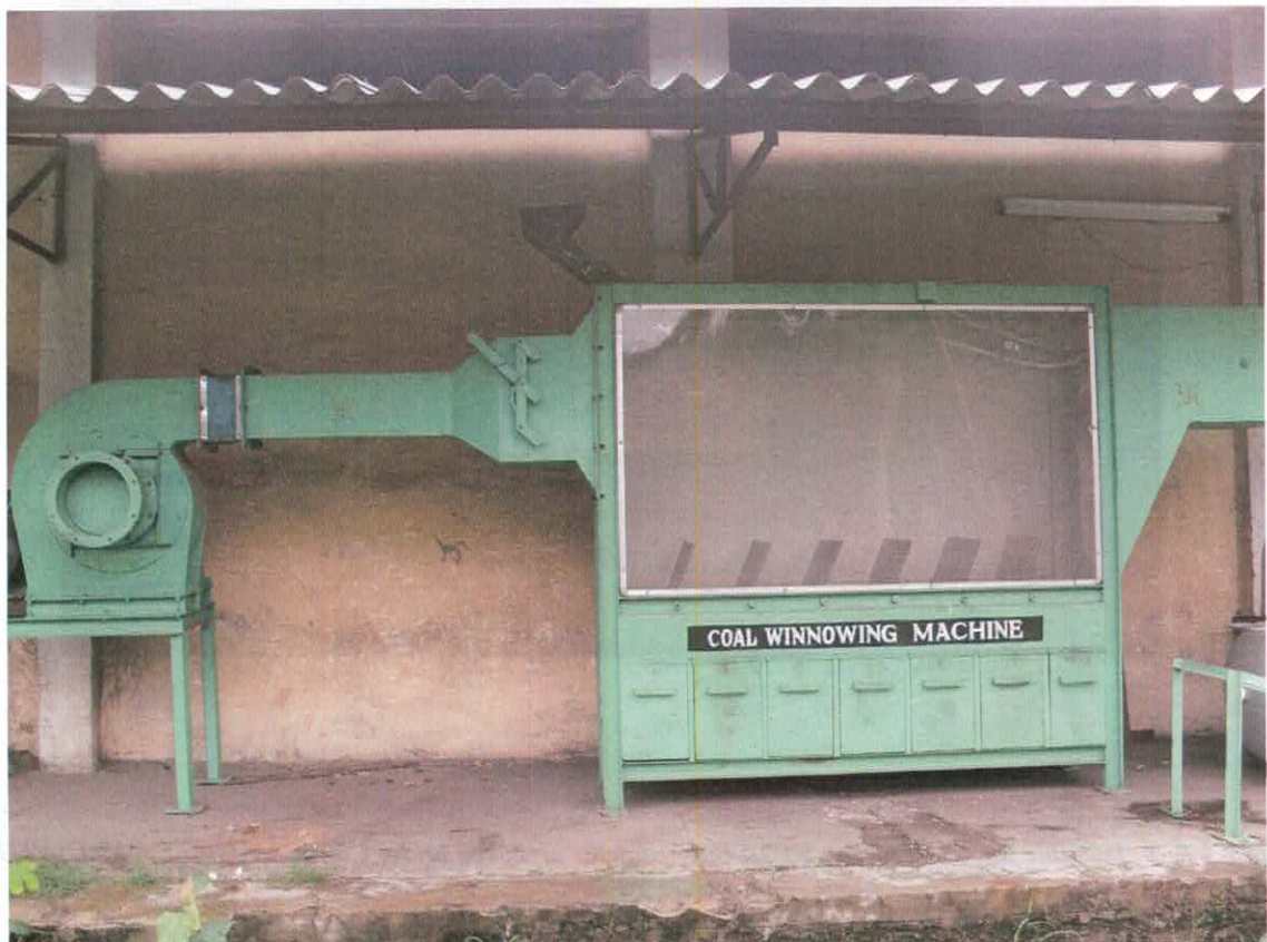
Lab Scale Coal Winnowing system developed under S&t Grant of MoC — CP/45
