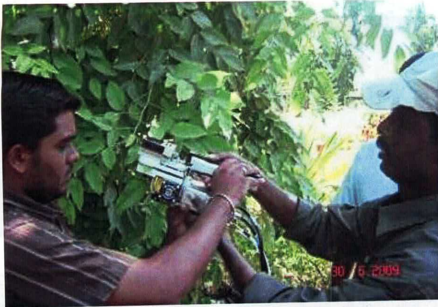
Measurement CO 2 absorption, conductance, transpiration rat, PAR etc with LICOR Analyzer at NLC Neyveli – EE/37
