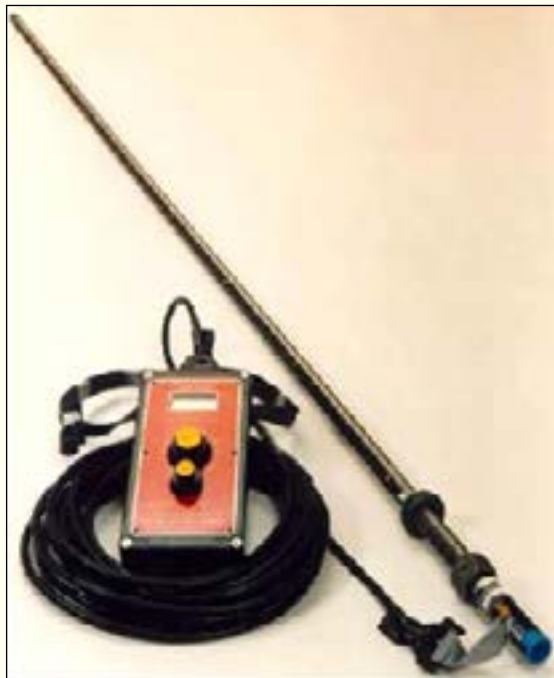
Fig.-8: Strain Gauged roof bolt
