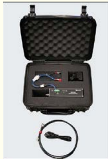
Fig.-35: Portable Time Domain Reflector cable into borehole to be filled with grout
