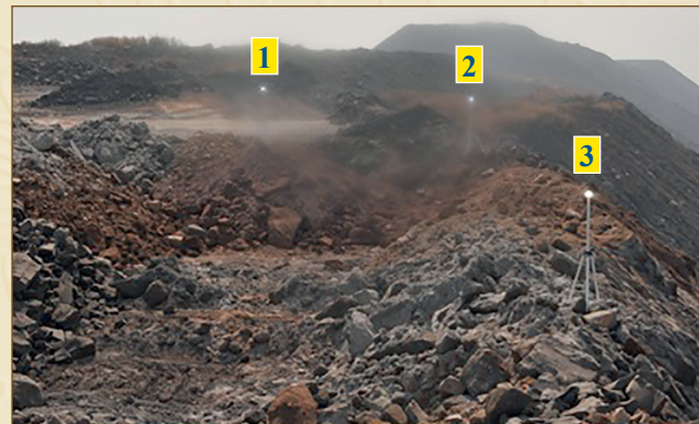
Retro-reflectors (Tiepoints) placed around the TLS
