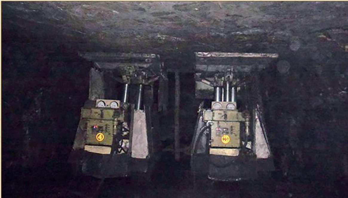
Fig.- 5: SAGES 3 & 4 installed at a Goaf Edge in Block B of Panel 2AN13
