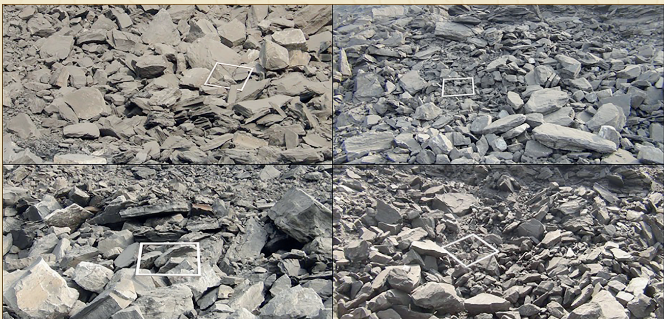
Photograph-1: A view of the blasted muck resulted in different experimental sites
