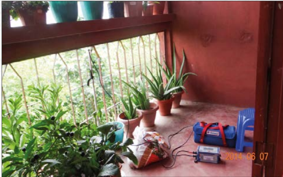
Plate-5: View of vibration monitoring point on 1st floor of an adjoining residential house at Ch: +400 m blasting location.
