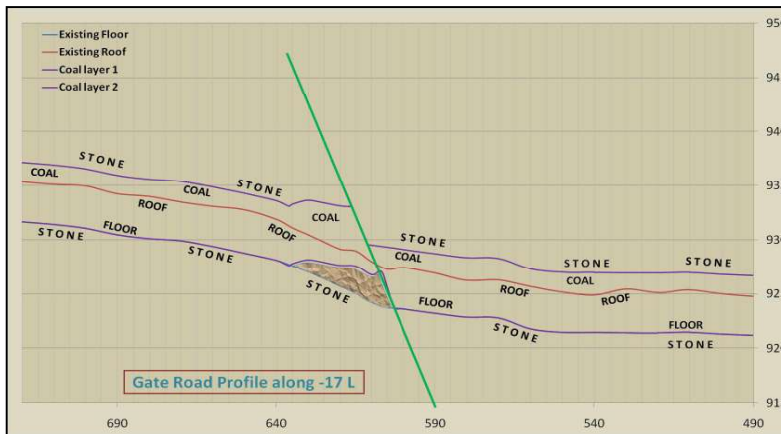
Fig.-6: Gate Road Section (Section B-B of Fig.4) and Stone Excavation during Development (-17L tail gate)
